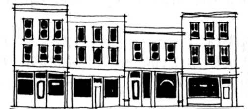
Examples of inappropriate storefront alterations. From left to right: new storefront features a “colonial theme” that is stylistically inappropriate; reflective glass prohibits pedestrian interaction with the storefront; storefront has been removed entirely and covered up with incompatible wall material and columns appear undersized and “weak.”
